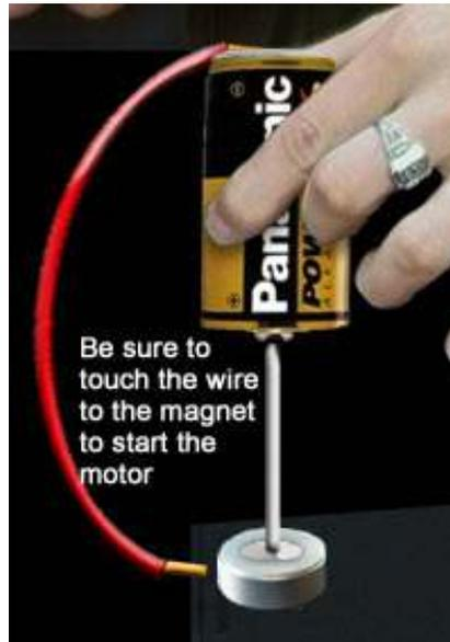
An extremely simple motor can be assembled from just a battery, a nail, a neodymium magnet, and a length of copper wire. The arrangement of these elements is shown in the image to the left.
