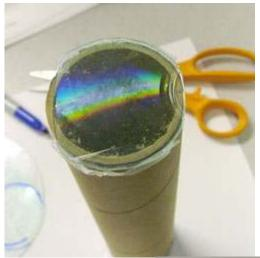
The circular grating is attached to the other end of the tube using household cement or hot glue. Before attaching the grating, make sure that the grating's grooves are parallel to the slit.
