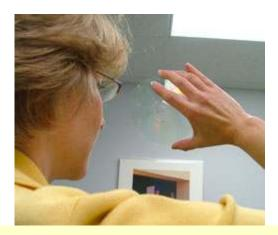
A clear CD-R may be used as a grating simply by holding it about 20 cm from the eye and centering the light source to be analyzed in the hole of the CD. A particular advantage of this type of spectroscope is that it may be used to study sources of low intensity such as an LED or the moon.
